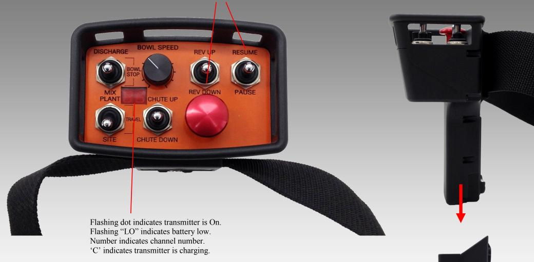
Stow transmitter in Base Unit Charger. Only install rechargeable batteries.
