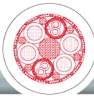
for flexible and fixed laying, 4 supply cores + 2 shielded pairs
