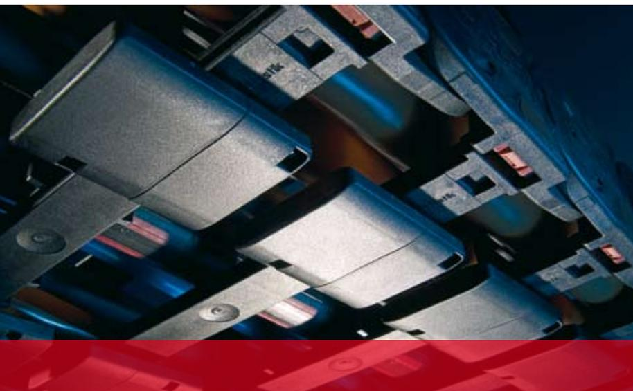
The ability to adapt the housing of the magnet holder (see illustrations) to the cable drag chains removes the need for special - and therefore expensive - components.
