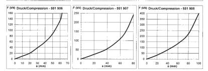
There is a possible deviation of approx. +/-20% in the above values due to production and hardness tolerances.
