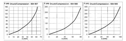
There is a possible deviation of approx. +/-20% in the above values due to production and hardness tolerances.
